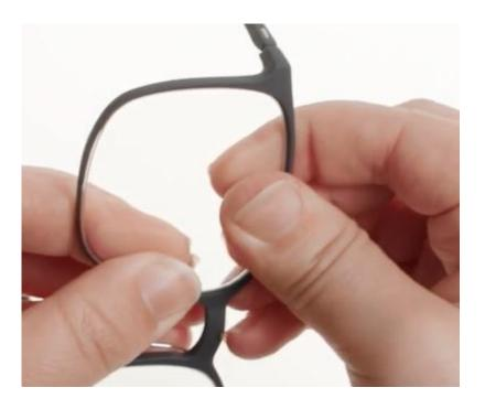
Continue inserting the lens along the top to the nasal side
