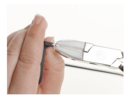
Adjust metal hinge double-padded plier in the desired direction Reinstall temple
