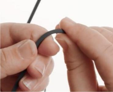
Adjust the temple end to the ear and head shape using large curves Do not put pressure on the temple tip when adjusting temple curve
